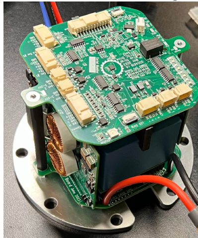
Unit pictured has 1000V-tolerant integrated logic supply
